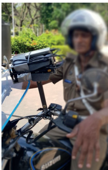
Fig. 2. Sniffer 4D sensor mounted on a police traffic motorcycle
