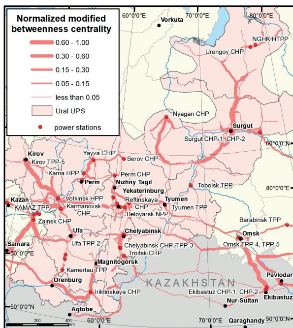
Fig. 7. Electrical grid centrality calculated using author's script
