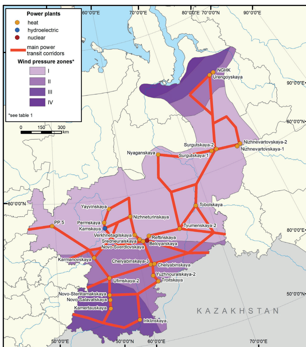
Fig. 4. The main power transits in the Ural UPS overlaid with the wind pressure zones
