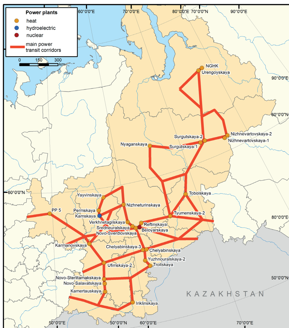
Fig. 1. Schematic map of the main power transits in the Ural UPS
