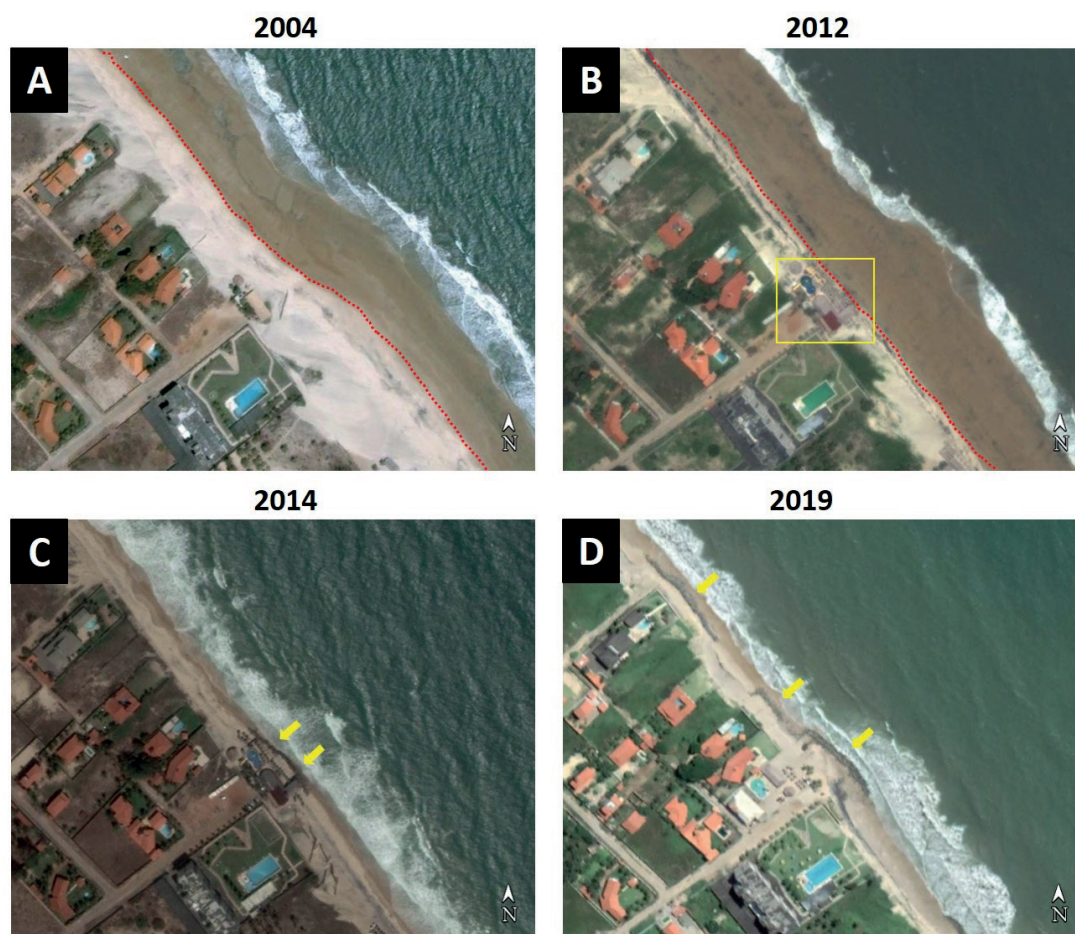
Fig. 5. A stretch of Tabuba Beach in different dates. A) in 2004, the edge between dry and wet sand (red striped line); B) in 2012, the yellow square indicate the place of a beach hut; C) and D) indicate the presence of rockfills (indicated by the yellow arrows) to contain the progress of erosive processes. Source: Google Earth
