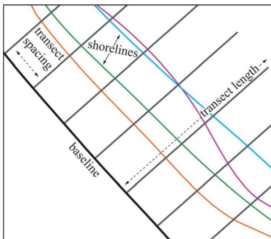
Fig. 3. Launching of transects from the baseline parallel to the shoreline vectors. Source: Thieler et al. (2017)
