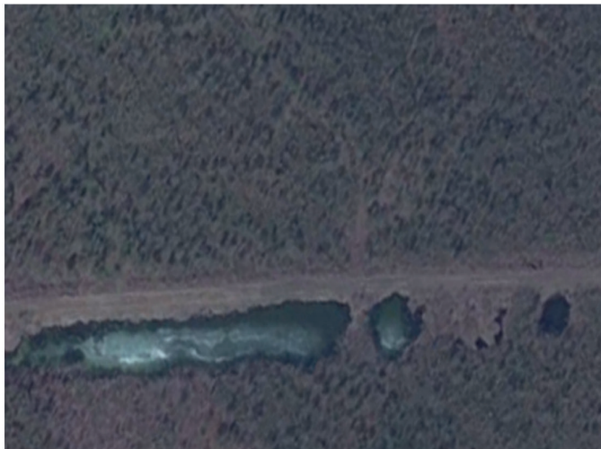
Fig. 1. (a, b). A typical remote sensing image of emerged thermokarst depressions along a road: a) high-resolution remote sensing data, GeoEye image b) photo
