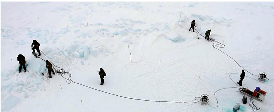
Fig. 2. General view of hot water ice drilling unit UVBL-2. The picture shows the operation of two drilling stations. In 2018, drilling of ice ridges was conducted using one station
