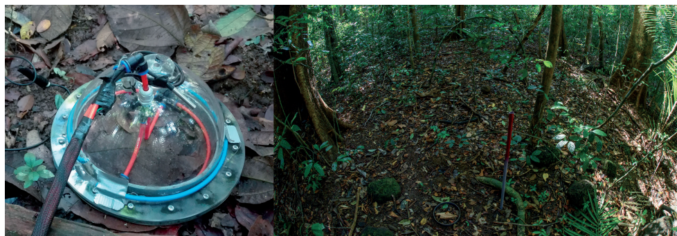
Fig. 3. Measuring chamber (left) and a collar at one of the sampling points (right)
