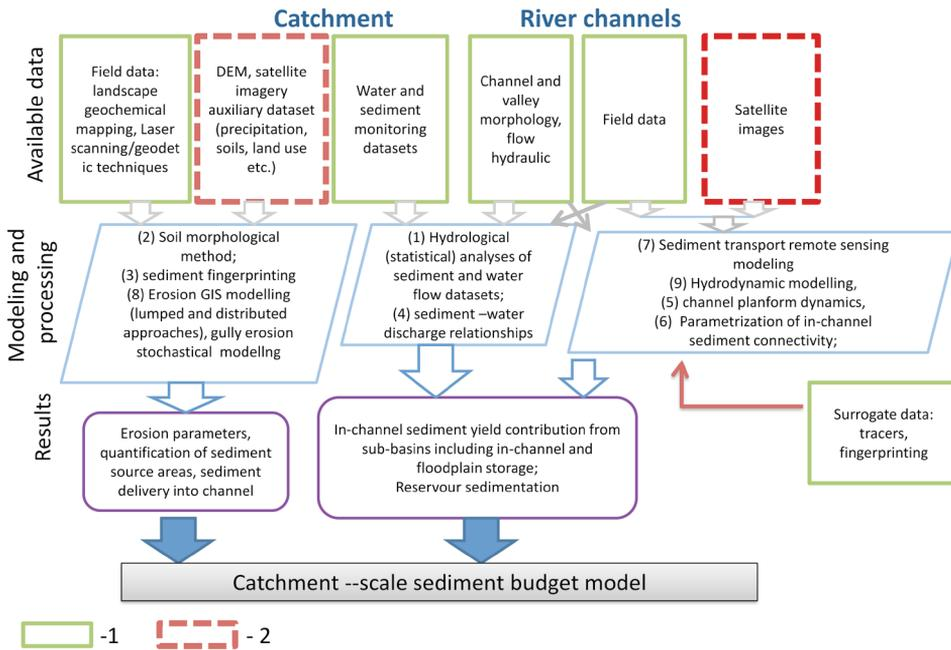
**Fig. 6. Conceptual framework of catchment sediment budget toolbox (1 – field-based datasets; 2 – GIS and RS datasets)**
