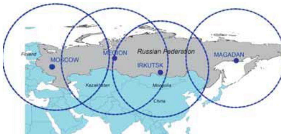
Fig. 11. Satellite imagery coverage in Russia and adjacent countries using UniScanT receivers (data from http://www.geogr.msu.ru/science/projects/geoportal )
