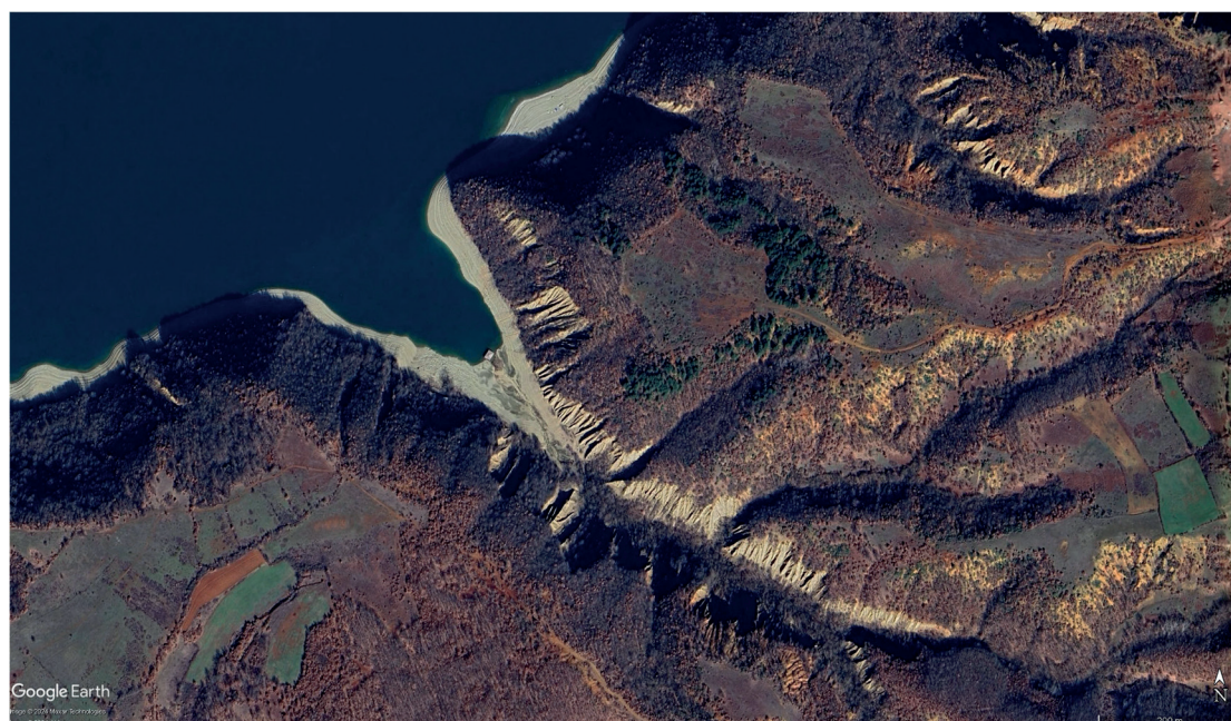
Fig. 3. Gully erosion and extreme erosive processes on the banks of the Spilje reservoir
