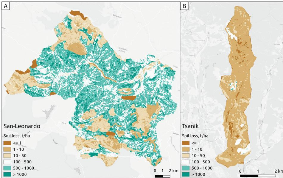
**Fig. 5. Application of erosion models for San-Leonardo (A) and Tsanik (B) river basins (net annual soil losses, t/ha)**
