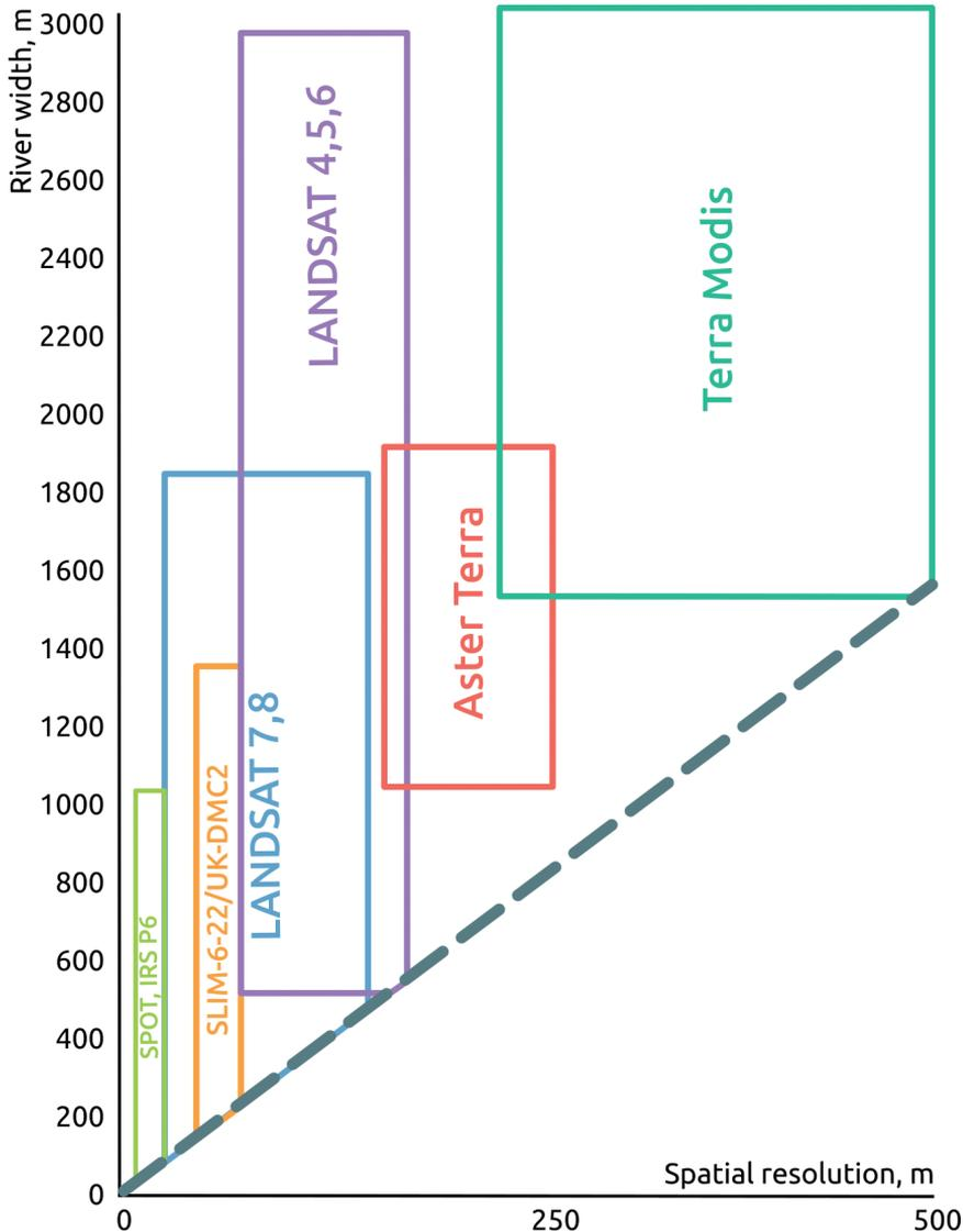
Fig. 4. Spatial limits of RS application in sediment concentration analyses
