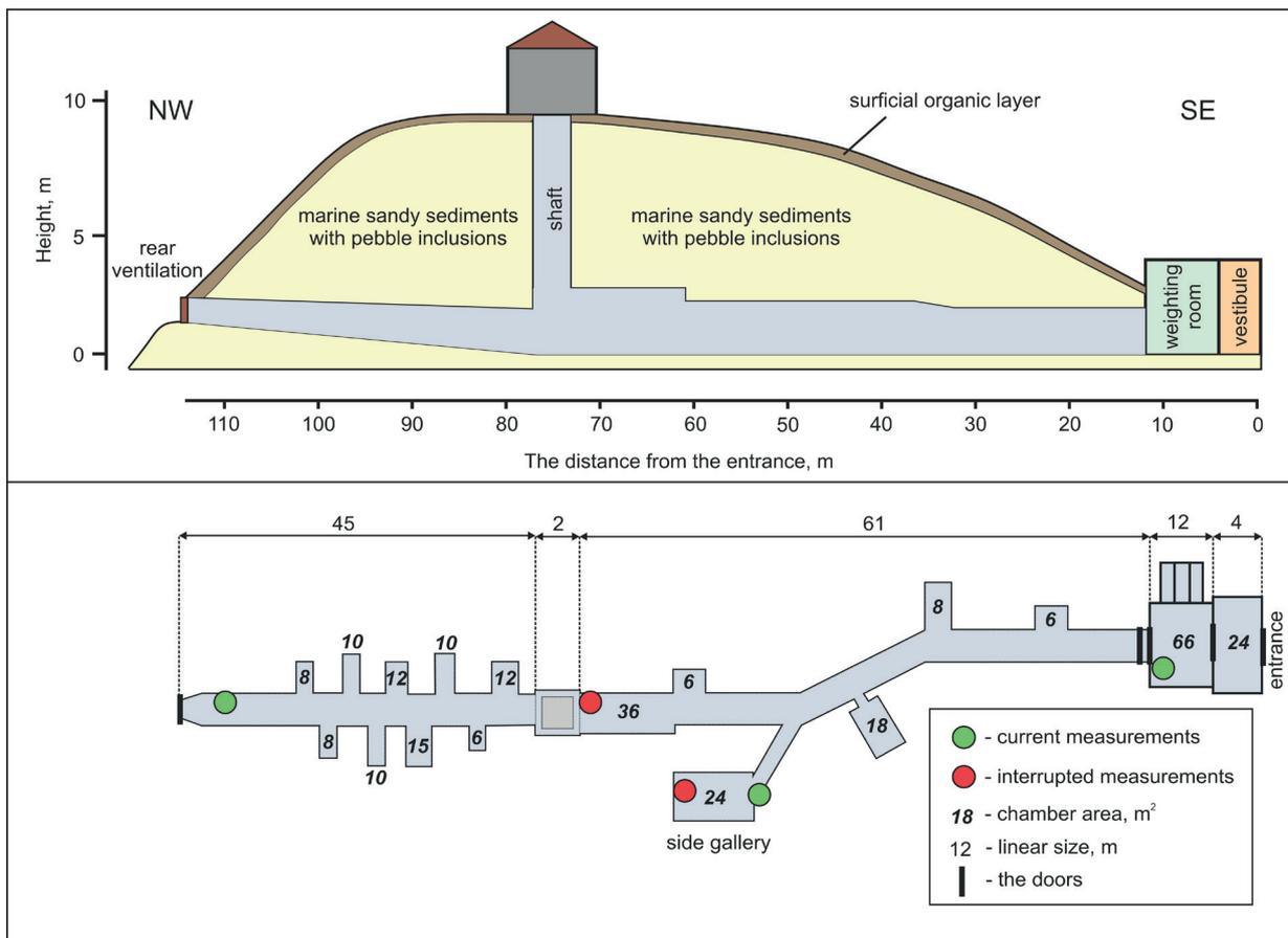
Fig. 2. Schematic of the Lorino community ice cellar (top) in cross section along the main gallery and (bottom) in plan view (source: field measurements in 2019)
