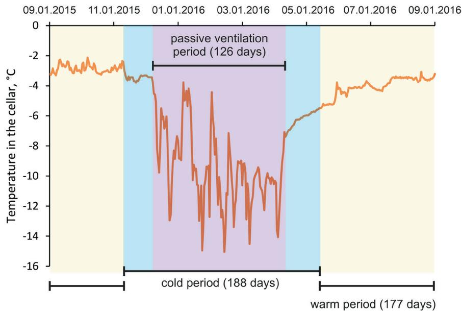
**Fig. 5. Daily temperatures in the Lorino community ice cellar from September 1<sup>st</sup>, 2015 to September 1<sup>st</sup>, 2016. Note the effectiveness of passive ventilation at lowering the internal ice cellar temperature through the summer of 2016, although summer average temperatures for 2015 and 2016 are -3.3° C and -3.1° C respectively**
