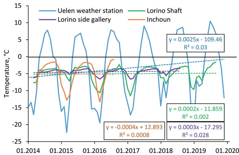
**Fig. 7. Monthly dynamics of internal air temperatures in the Lorino and Inchoun ice cellars and at the Uelen weather station from 2014 to 2019.**
